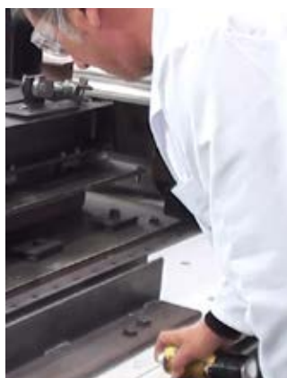
Figure 4: Spray release agent on the surfaces of the U-profile
