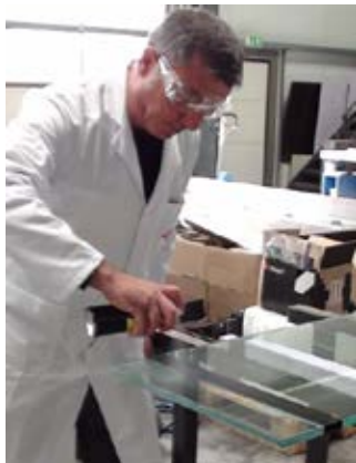
Figure 3: Spray release agent on glass
