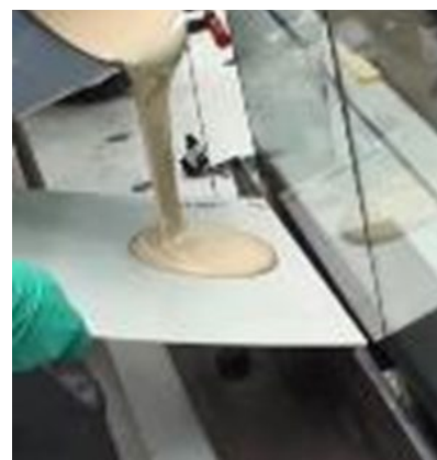
Figure 13: Using guiding plate method to fill U-profile with glass embedding material
