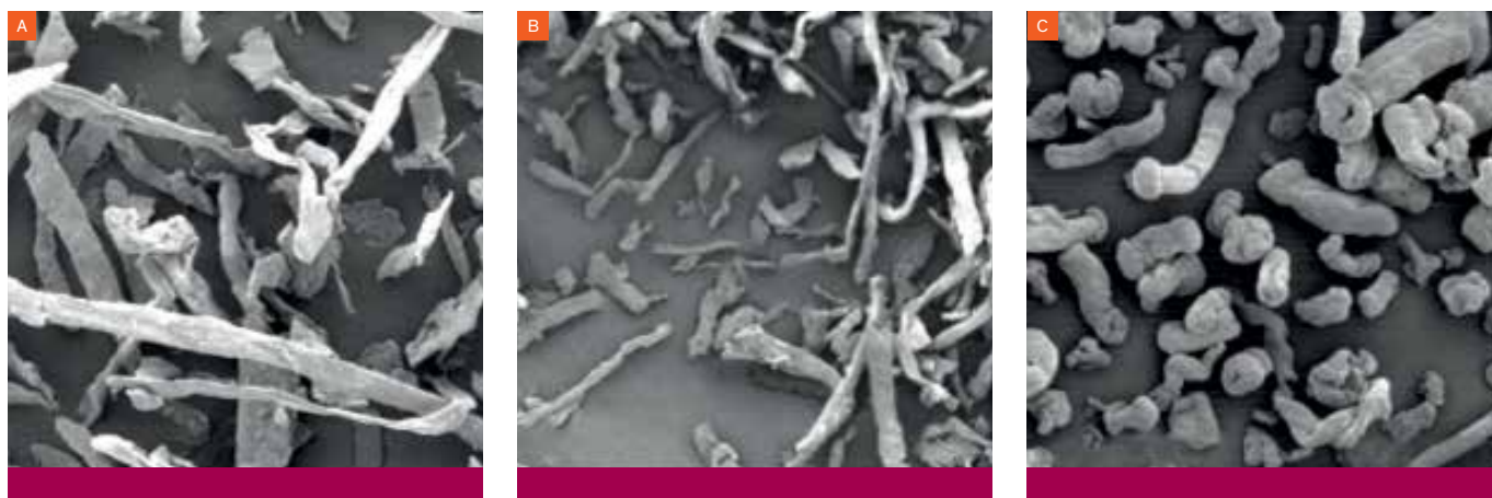
Figure 03: Three scanning electron microscopy pictures of cellulose (A) and cellulose ether with regular (B), and optimized particle morphology (C)
