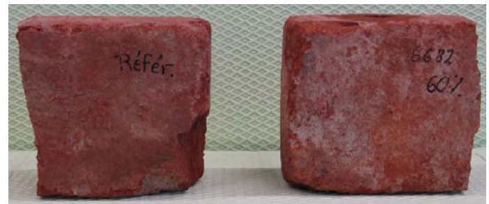
Figure 7: Optical and infra-red photography of bricks treated with silane emulsion diluted at 60% or 7.5%. Pictures were taken after the bricks were placed in water bath to allow capillarity rise and left at RT for a couple of hours.
