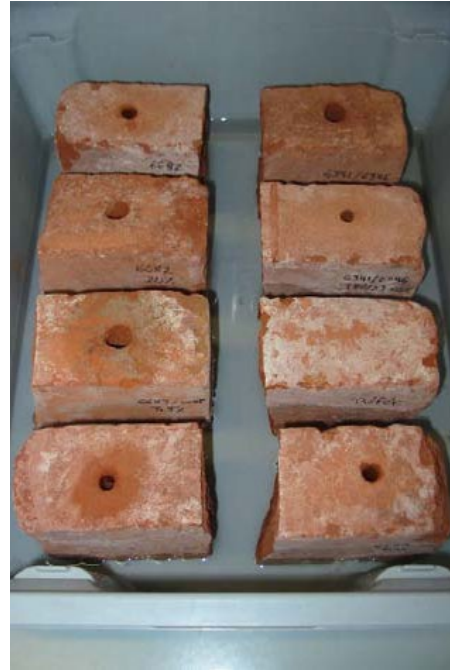
Figure 6: Water uptake of clay bricks injected with DOWSIL™ IE 6682 Emulsion @ 60% or 7.5% as a function of immersion time. Picture showing the experimental set up to measure water uptake by capillarity rise.
