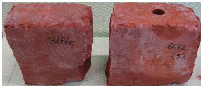
Figure 7: Optical and infra-red photography of bricks treated with silane emulsion diluted at 60% or 7.5%. Pictures were taken after the bricks were placed in water bath to allow capillarity rise and left at RT for a couple of hours.
