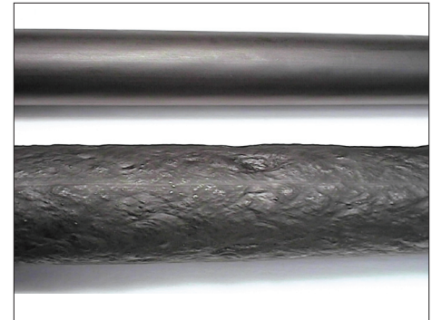
Scorch-resistant technology in SI-LINK AC (as shown in the upper cable) improves the insulation surface quality and appearance and reduces scrap.
