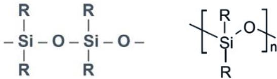
Figure 4. Silicone molecular structure
