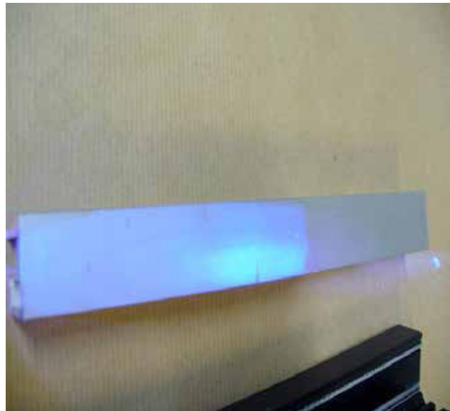
Figure 5: DOWSIL™ 1200 OS Primer or DOWSIL™ Primer-C OS is applied by cloth wiping onto the substrate. With proper UV lamp which can help the QA inspector visually check the correct application of the UV traceable priming.
