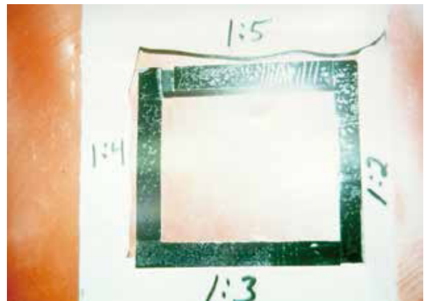
Figure 11 indicates Structural Bite: Glueline Thickness from 1:2 (right) to 1:3 (bottom) will allow for ease of access to ensure a complete joint fill. The poor joint fill for 1:4 & 1:5 can be seen in the above figure.
