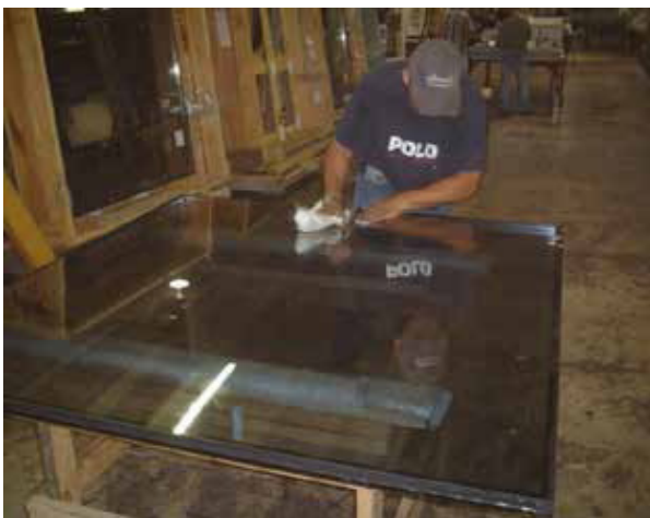
Applicator demo two-cloth cleaning method
