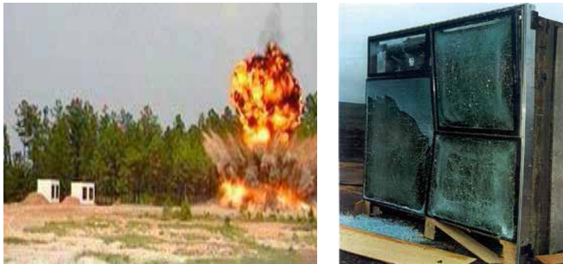
Figure 24: Protective Glazing bomb blast test photos (left) Glass units after Bomb blast testing in UK (right)
