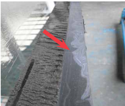
Sealant poor mixing (white streaking pattern) found in the deglazed units.
