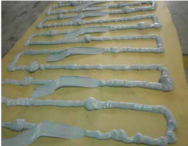
Snake test to help identify if pump mixing quality is consistently good or not
