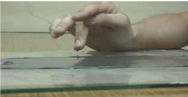
Sealant not formed skin yet hence will adhere to finger.
