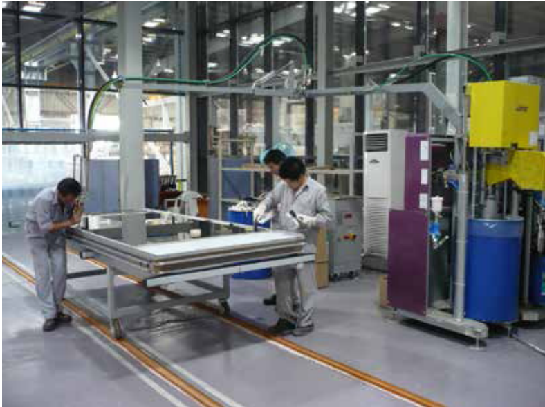
Figure 2: Two-component sealant (i.e. DOWSIL™ 983 Structural Glazing Sealant or DOWSIL™ 993N Structural Glazing Sealant) requires (adequate air-seal dispense) specialized dispensing equipment to mix the material prior to use. Application is usually limited to factory applied environments.
