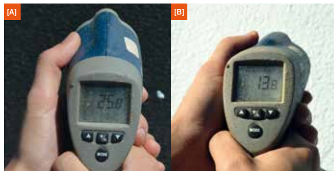
Outdoor temperature: 19°C [A] Bitumen temperature: 25.8 °C, [B] Cool Roof temperature: 13.8 °C
