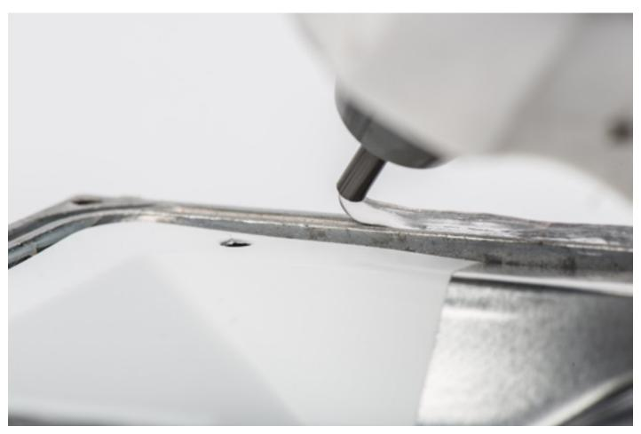
Hot-melt, neutral-cure sealants are intended for assembly, bonding, sealing, gasketing and other OEM applications that require instant adhesion and high green strength.
