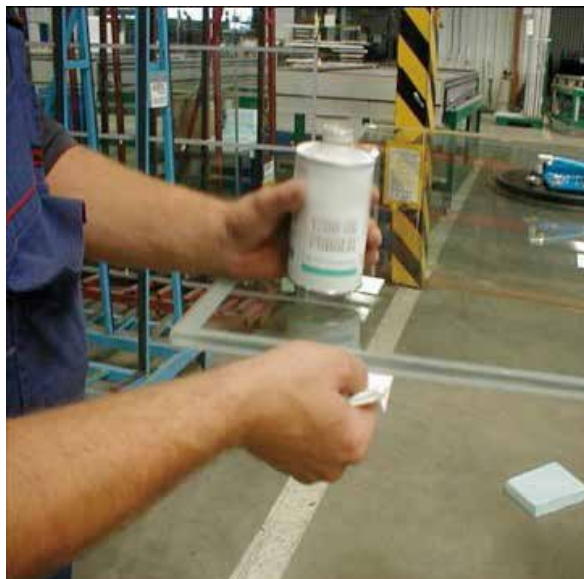
Figure 5: DOWSIL™ 1200 OS Primer or DOWSIL™ Primer-C OS is applied by cloth wiping onto the substrate. With proper UV lamp which can help the QA inspector visually check the correct application of the UV traceable priming.
