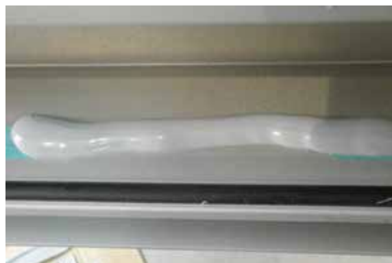
Photo left hand side demo a daily adhesion test performed on the off cut aluminium frames, right hand side photo shown a sealant bead applied onto a hidden area of glazed unit for verifying adhesion can be build up or not.
