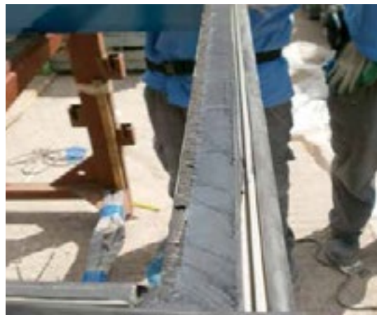
After structural joint cut open the un-glazed glass can be removed from the support frame. Right side photo shown the glass was removed then the joint fill (right photo showing excellent joint fill) and sealant mix quality can be visually check.
