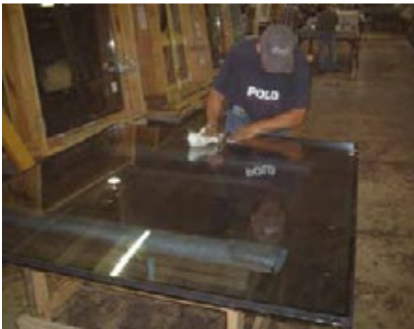
Applicator demo two-cloth cleaning method
