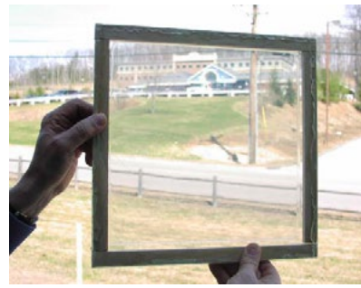
Figure 7 – Highly transparent aerogel interlayer system (Courtesy of Aspen Aerogels)
