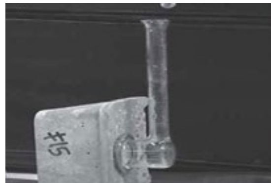
Figure 1: Rilem Tube Test for Water Absorption
