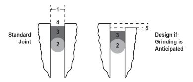
Figure 2: Recommended Joint Designs.
