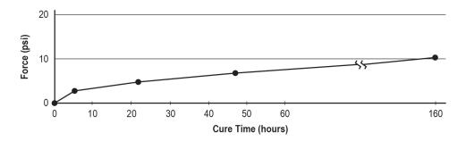
Figure 1: Cure Rate of DOWSIL™ 902 RCS Joint Sealant.1
