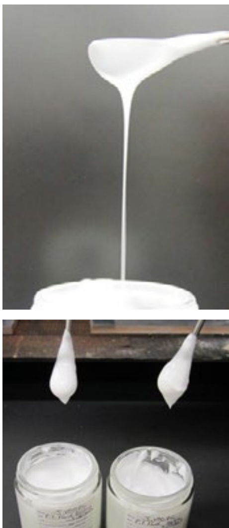
Picture 1: Stringy texture provided by the branched silicone polymer (top) in comparison with creams with silicone gums and silicone elastomers.
