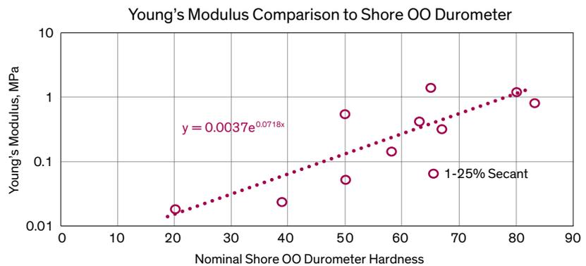
exponential curve fit also appears to fit very well to the data. Again, the DMA derived modulus is significantly higher than that from stress/strain curves (there was not enough RDA data available to plot).
