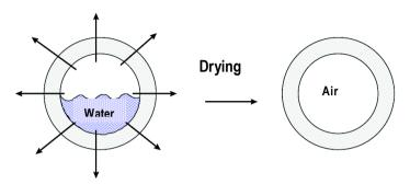
ROPAQUE™ Opaque Polymers have a narrow particle size distribution and are similar in size to TiO2 particles. This allows them to act like ultra-fine inorganic extenders, spacing TiO2 effectively and therefore increasing its efficiency as a primary pigment.
