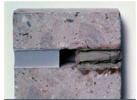
DOWSIL™ Silicone Sealant and a leading polyurethane sealant after 2,500 hours of humidity and UV exposure in extended weathering, heat and stability tests
