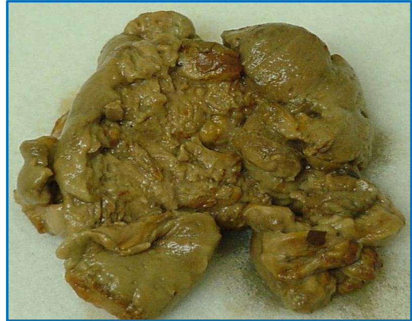
Bio-fouling - customer sample with 11% propylene glycol
