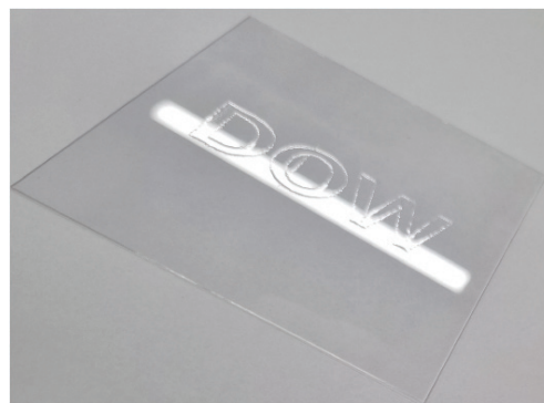
Example of inkjet printing with a Konica Minolta KM1024MHE/14PL printhead on glass without surface treatment.
