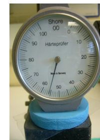
DOWSIL™ TC-4525 Gap Filler Cure Rate: Hardness Evolution at Different Temperatures
