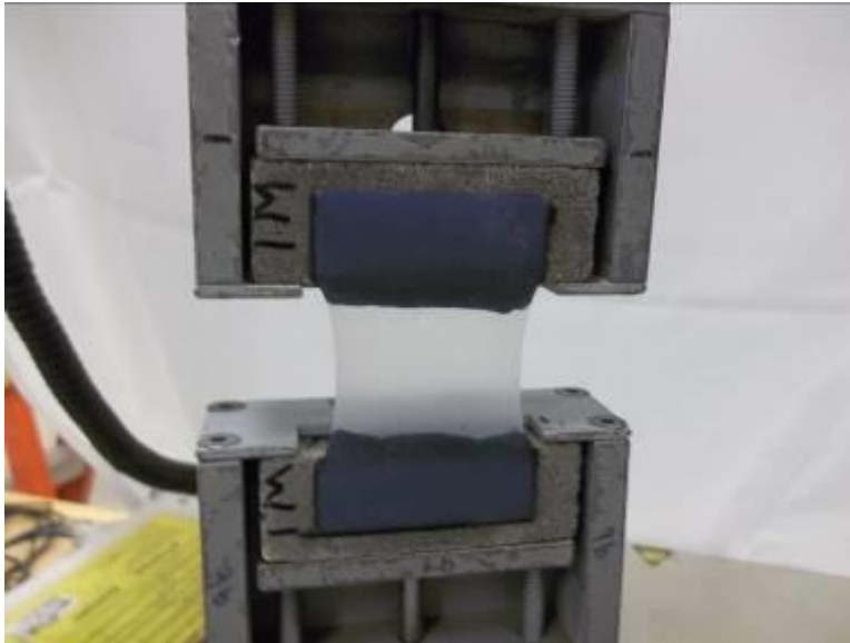
Photo No. 11 ASTM C1523 Water Immersed Unmodified Specimen During 1-Hour Hold Cycle Detail (Typical)
