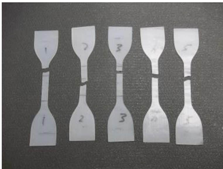
Photo No. 4 ASTM D412 Specimens Failure Detail (Typical)
