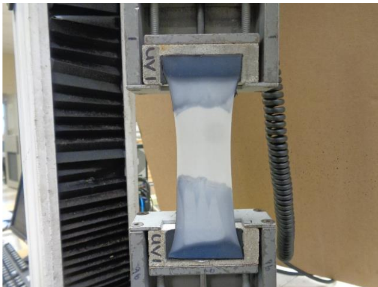
Photo No. 22 ASTM C1523 UV Weathered Unmodified Specimen During Breaking Strength (Typical)
