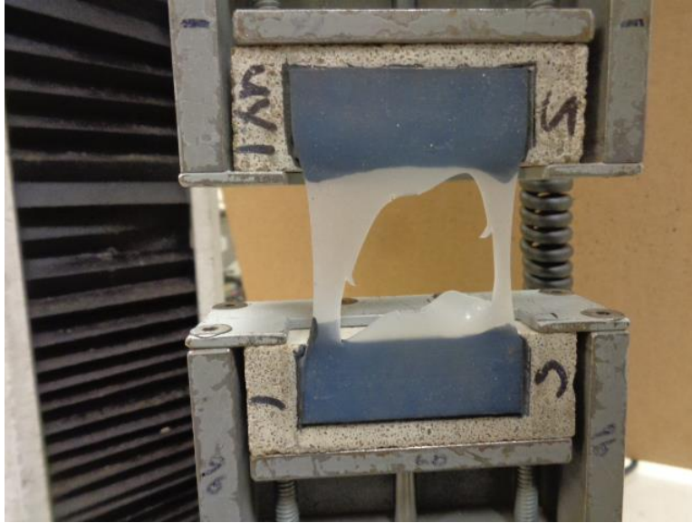
Photo No. 21 ASTM C1523 UV Weathered Modified Specimen During 1-Hour Hold Cycle Detail (Typical)
