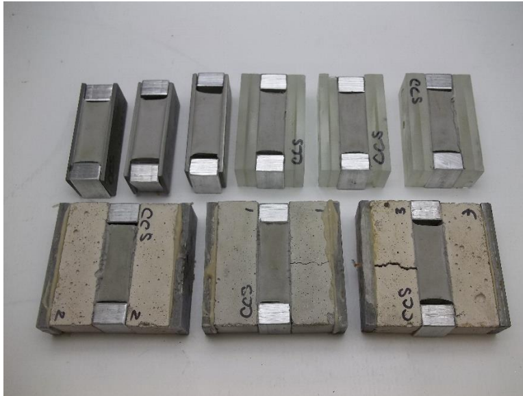
Photo No. 3 ASTM C719 Specimens Post-Test Detail (Top)
