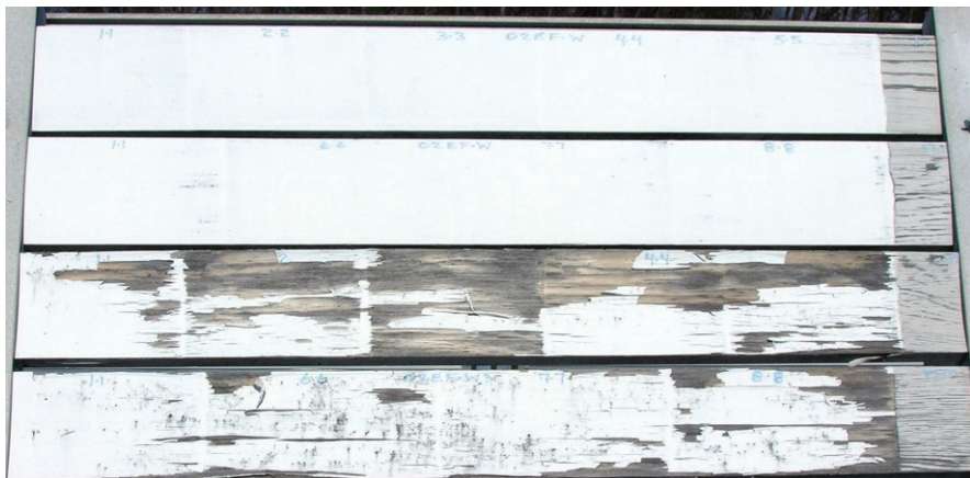
FIGURE 8—A comparison of panels prepared from fresh white pine (two boards on top) and white pine weathered for three months before coating (two boards on bottom). Panels were coated with the identical series of paints and exposed for two years in a south 45° orientation in Spring House, PA.
