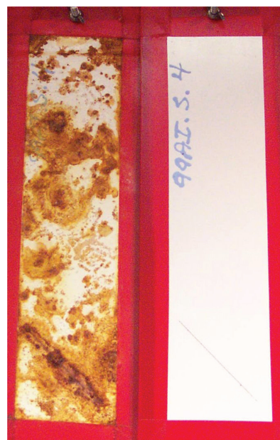
FIGURE 6—Cold-rolled steel panels coated with the same waterborne acrylic direct-to-metal coating and exposed south 45° at Sea Isle City, NJ, (left) and Spring House, PA, for two years.
