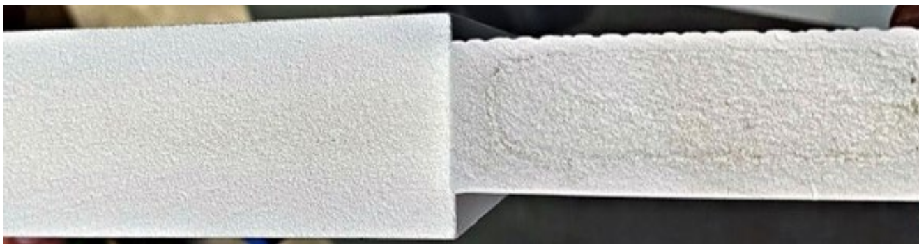
SURECEL™ T-60 process aid (left) provides unmatched cell structure at thickness >1”.
