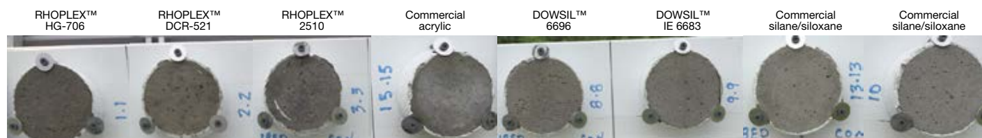
Natural look concrete sealers exposed 12 months North vertical on 7 day cured tilt-up concrete substrates in Spring House, PA (Series 18ED)
