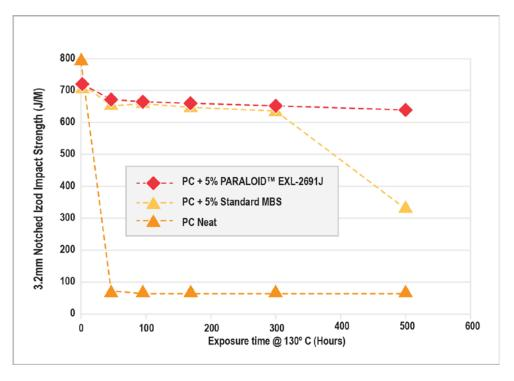
Thanks to its special stabilization package, PARALOID™ EXL-2691J IMPACT MODIFIER displays unrivalled stability under certain abusive moulding conditions, allowing it to be used in several demanding applications.
