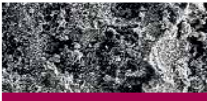
Figure 04: Cross section, uncoated weathered / Built-up roof surface 300X
