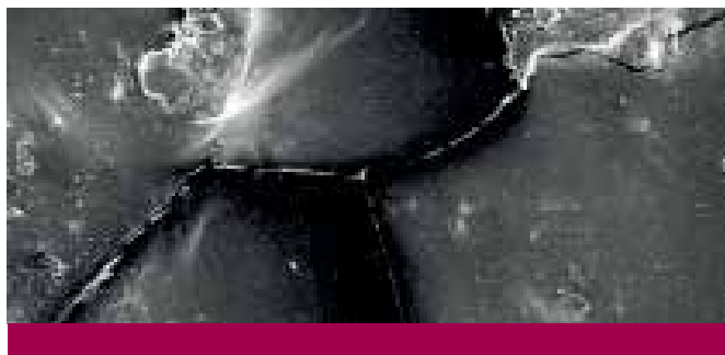
Figure 05: Cross section, coated weathered / Built-up roof surface (coating removed) 300X
