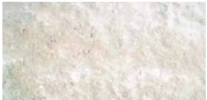
Soil treated with PAVECRYL after six hours of application. Soil is more compact, with a high degree of fine particle agglomerates.
