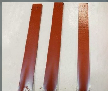
UL 94 flame bars, showing vertical burn orientation.
