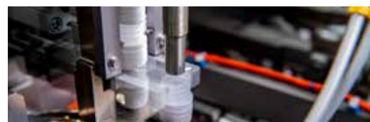
The Mespack HFFS line automatically pre-heats, inserts, and seals fitments for liquid packaging. Customers can examine packages within seconds to check every important detail. And make critical adjustments if needed within minutes.
