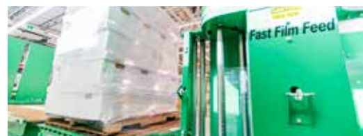
An industry-standard wrapper can test film characteristics coming off the roll, view wrapping interaction with loading formats, check wrapped layer requirements, and more.
