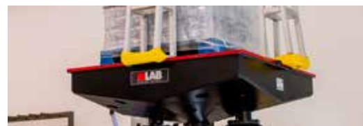
Pallets up to 3,000 pounds can be subjected to powerful vibrations to test against real-world encounters such as rough roads.
