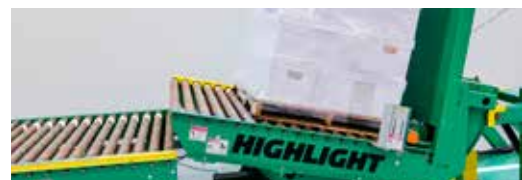
The transport simulator subjects wrapped pallets to real-world load stability challenges against rapid acceleration, sudden stops and impacts, and even tilt testing.
