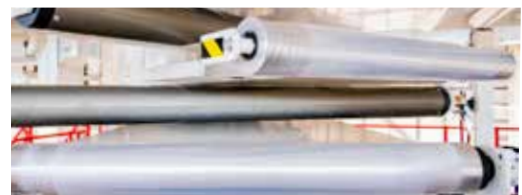
This is precision film making. Ideal physical properties, gauge profile, and consistency are maintained through multiple sensors from start to finish, including a 360-degree rotating nip.
