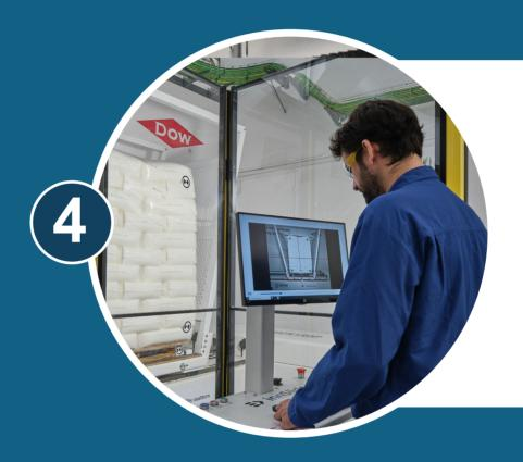
Load stability tests validated the films' performance in close-to-real transportation conditions and in accordance with the international quality standards, such as EUMOS 40509 and the US FMCSA Cargo Securement Requirements,
