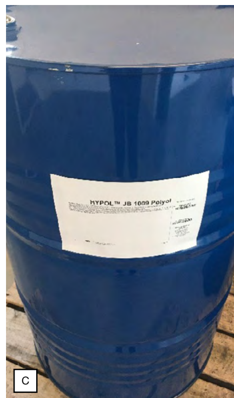
C: HYPOL™ JB 1009 Aqueous liquid formulation (Phase B) is supplied to OEMs packaged in blue phenolic lined 55-gallon drums.
