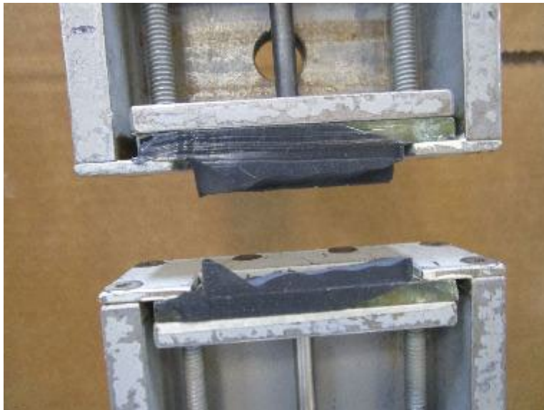
Photo No. 4 ASTM C1135 - Tensile Adhesion - Test Failure Detail
