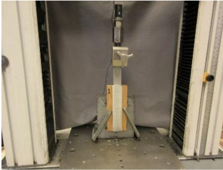
Photo No. 3 Adhesive Strength Test Setup
