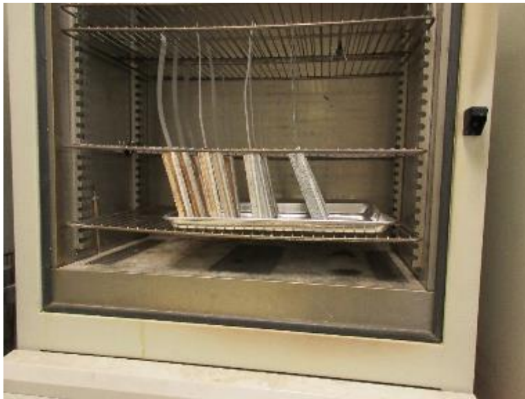
Photo No. 13 Specimens During 7 Day Level I Conditioning
