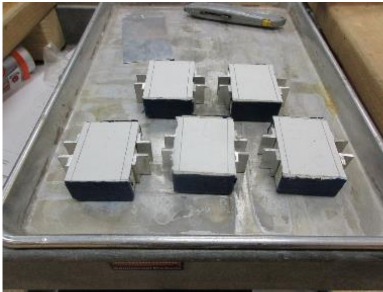
Photo No. 19 Crack Bridge Specimens Prepped. (Section 5.6)
