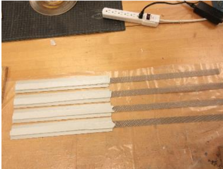
Photo No. 23 Prepped Specimens for Water Immersion (Section 5.7)
