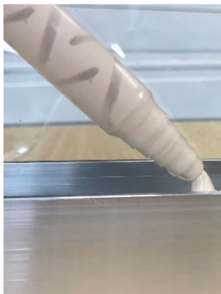
Figure 10: Injecting the mixed Part A and Part B in the U-profile
