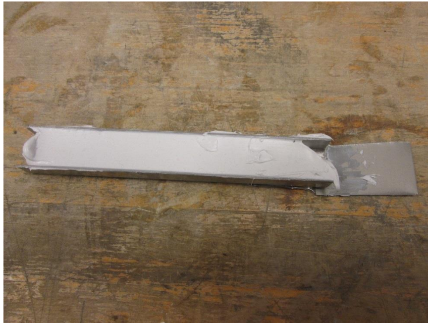
Photo No. 1 Typical Rheological Flow Test Specimen
