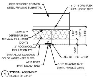
Unitized exterior cladding panel construction includes Dowsil™ DefendAir 200 as its vapor-permeable protection.
