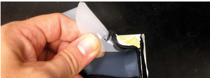
Figure 3: Tab adhesion test procedure
