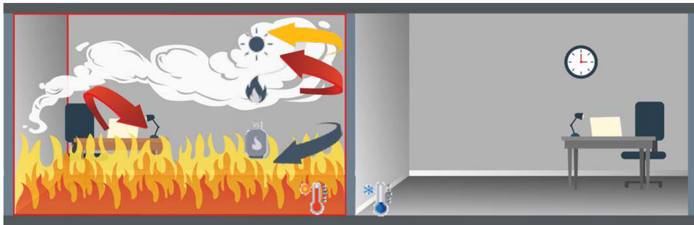
Figure 11: Compartmentation in buildings: fire rated walls and floors prevent the spread of fire (flames, hot gases and smoke) to adjacent rooms
