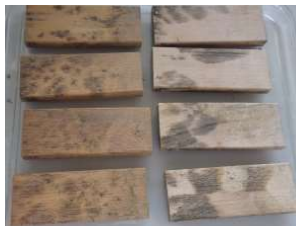
Figure 2: Blue stain growth on beech samples treated with water soluble silane (on the left) and untreated (on the right).
