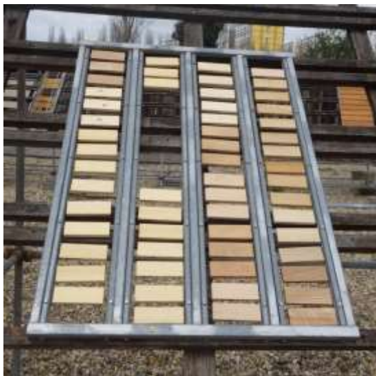
Figure 1: Specimens treated with the three silicon-based solutions and exposed outdoor.
