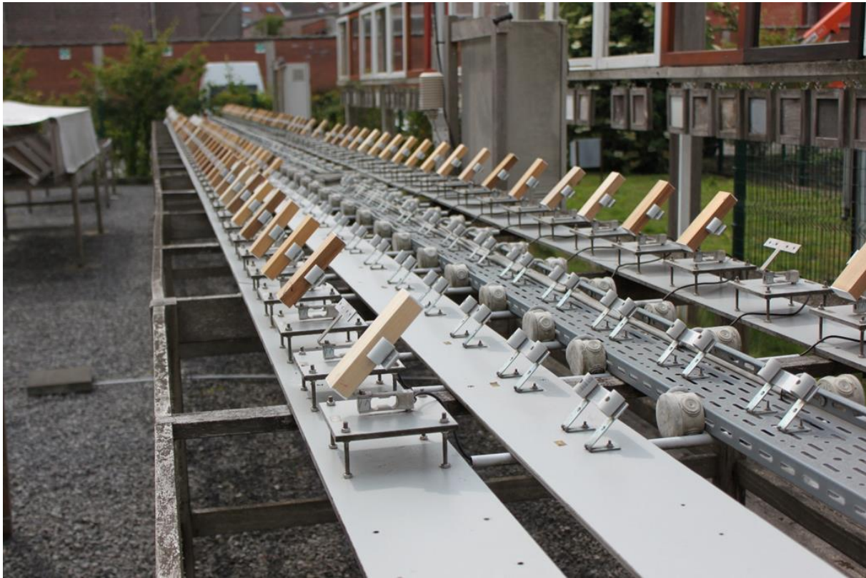
Figure 1: The continuous moisture measurement (CMM) set up.
