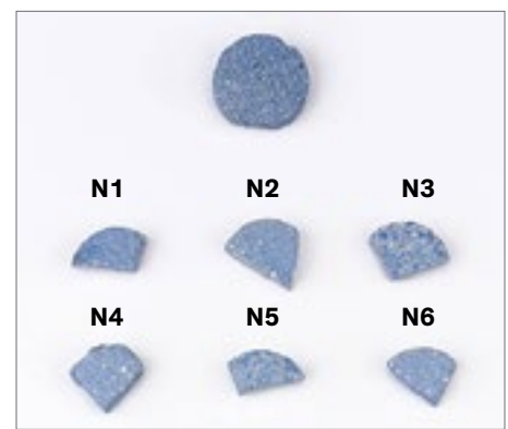
External surface of samples following 2 years of outdoor exposure in Barcelona.
