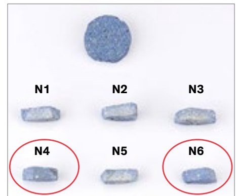
External surface of samples following 2 years of outdoor exposure in Barcelona.
