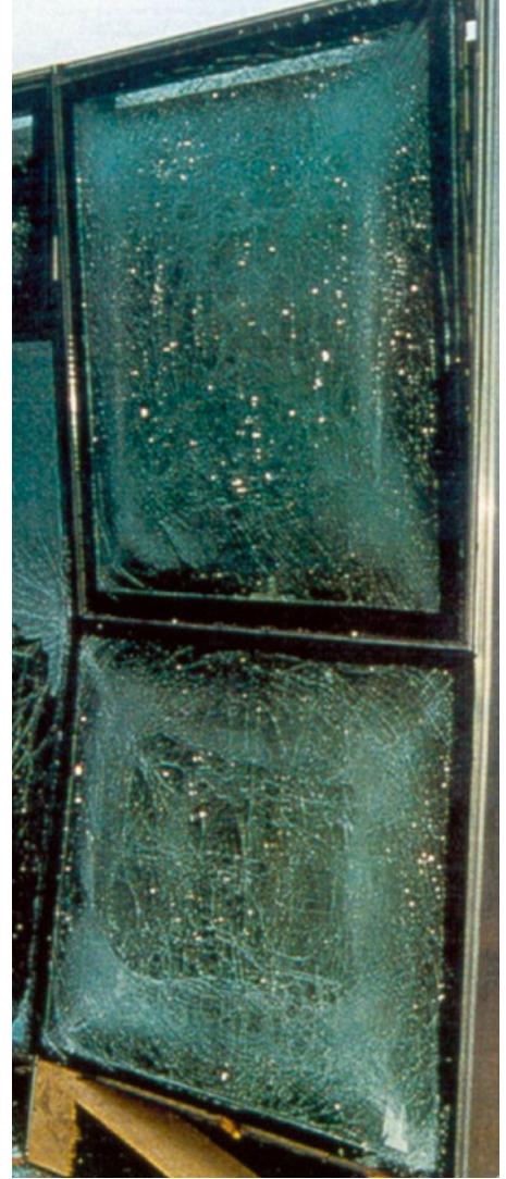
In controlled bomb-blast application testing conducted by Dow, 12 kilos of TNT were exploded 6.5 meters away from a 12 x 12-meter glass curtainwall panel structurally glazed on all four sides with a DOWSIL™ Silicone Structural Glazing Adhesive/Sealant. While the glass broke during the explosion, the facade stayed largely in place, thanks to the strength and flexibility of the sealant.
