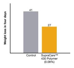
Rate of wear measured by the weight loss of bars after four days. NSD bars used a model formulation, with and without SupraCare<sup>TM</sup> 430 Polymer.
