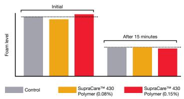
Normalized foam level: initial and after 15 minutes. Test conducted with a leading manual laundry detergent.
