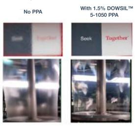
Data acquiried on monolayer blown film line using 1.5% PPA blended with LLDPE resin (octene coploymer, 0.5 g/10 min). Extruder parameters include melt temperature of 480°F, L:D Ratio of 14 and apparent shear rate of 300/s at 45 min.
