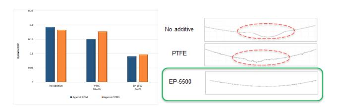
DOWSIL™ EP-5500 Powder long term dynamic coefficient of friction measurements under different conditions:
