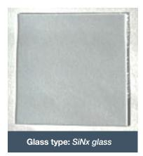
**Test condition**: 85°C/85% 240h reliability test
