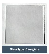
**Test condition**: 85°C/85% 240h reliability test
