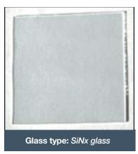
**Test condition**: 85°C/85% 240h reliability test
