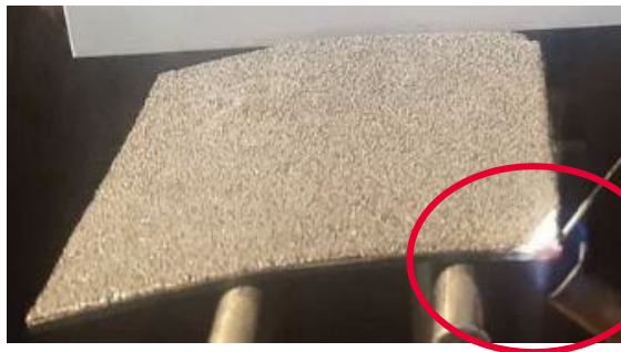
Flammability test on 3mm-thick DOWSIL™ 3-6548 Foam
